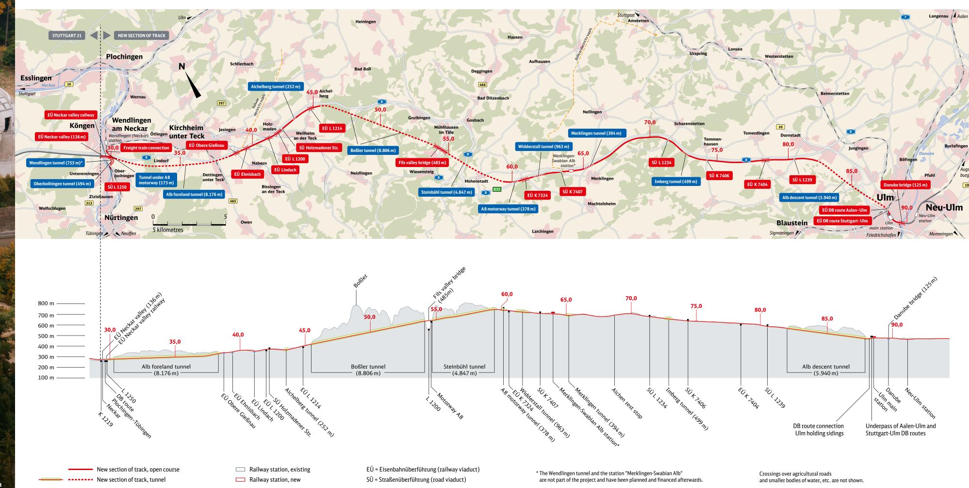
Covering a distance of roughly 60 kilometres, the new Wendlingen-Ulm section belongs to Deutsche Bahn's high-speed network and is part of the Stuttgart-Ulm Rail Project.
